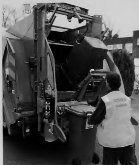
Barnet's domestic refuse is collected using 26 tonne Refuse Compaction Vehicles
