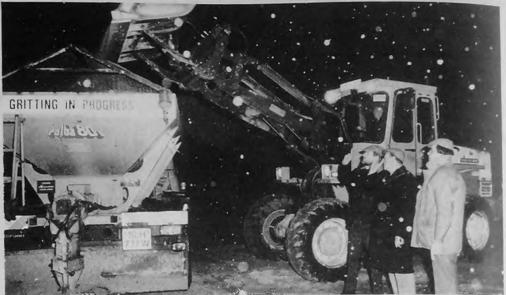
At the Squires Lane depot salt is loaded into one of the purpose built gritters to help keep the roads clear during last January's bitterly cold spell.
