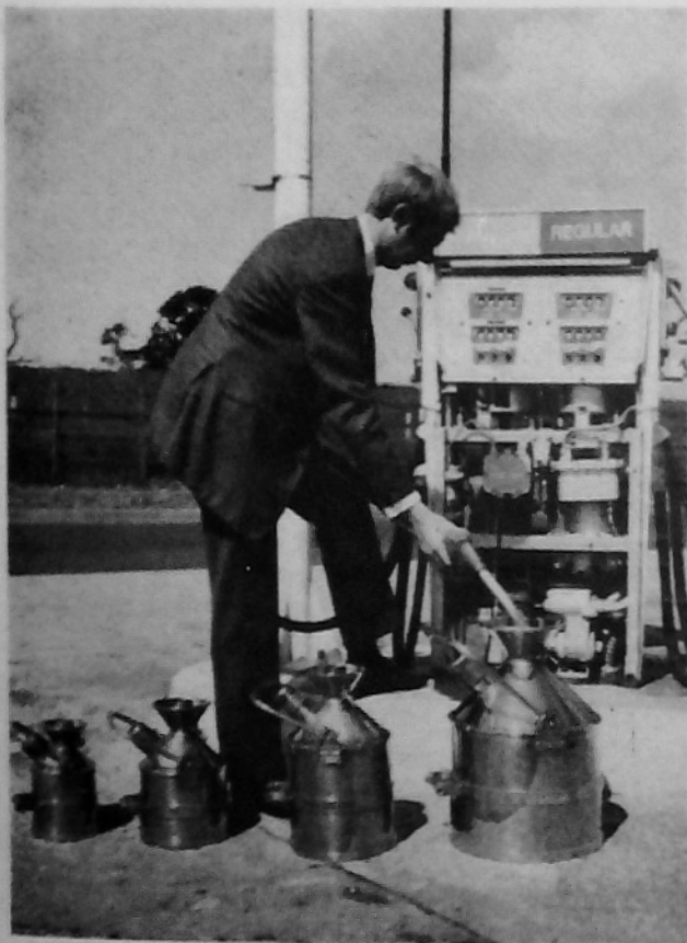
A petrol pump being tested for accuracy prior to being sealed by the Inspector.
