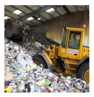
The tipping floor at a MRF. Incoming materials are received and stored here prior to processing.
